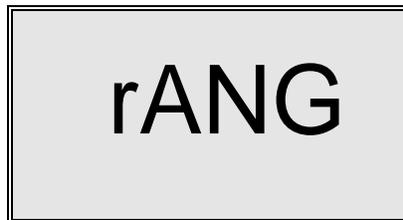
The length of the range search depends on the number of ranges which must be searched in order to find the correct range for the sample. During the range search, the instrument will appear to freeze on a given reading for a few seconds then, once the range is located, will pinpoint the exact reading on the display. The display may also switch to **00.0** for a second or two during a range search before it selects the proper range.
